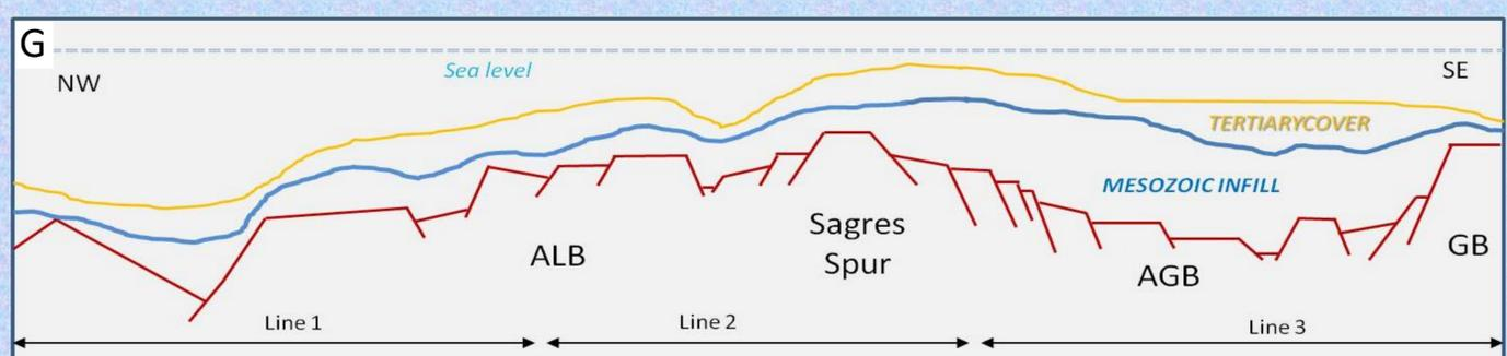
**G** – Sketch of the basement structures and Meso-Cenozoic infill of the Alentejo Basin (ALB) and Algarve Basin (AGB), based on the composition of three interpreted seismic lines (vd. Fig. B for location). ALB – Alentejo basin; AGB – Algarve Basin; GB – Guadalquivir Bank.
